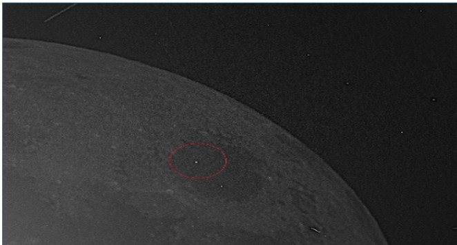
Figure 1: Maximum-stacked lunar image obtained from a sequence of registered frames. Numerous point-like and linear artifacts caused by hot pixels and cosmic ray events are visible, while a localized transient consistent with a lunar impact flash is clearly detectable in the Mare Crisium region. A slight high-pass filtering has been applied for Clarity.
